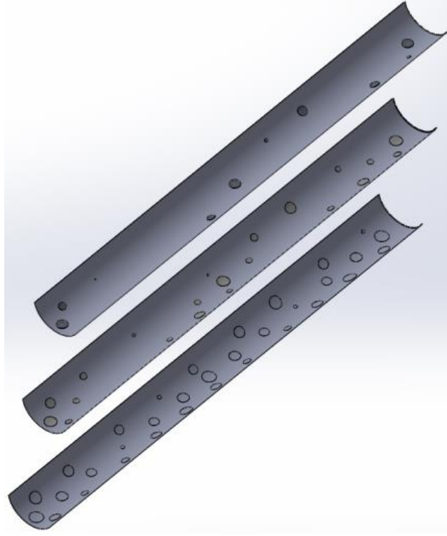
Figure 6.9. MPL carbon particles in contact with a GDL fiber: Increasing compression ( F < F' < F'' ) increases the number and contact area of Hertzian contact ellipses (the size of particles and contact areas have been exaggerated for clarity)
