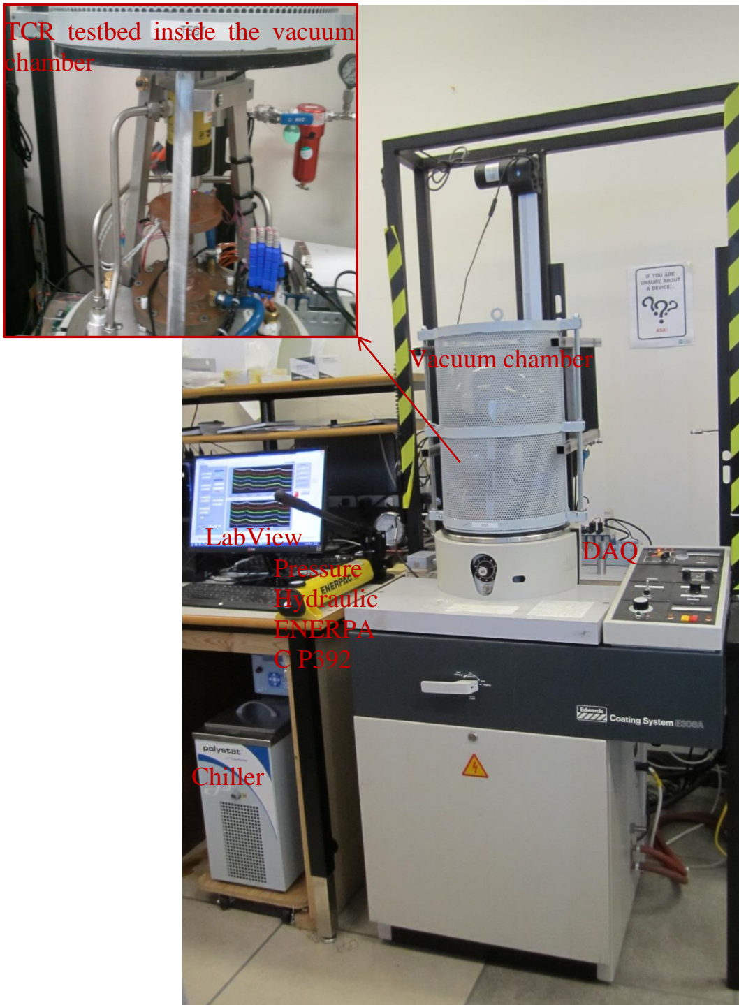
Figure 3.1. Thermal conductivity and contact resistance apparatus (TCR machine)
